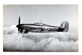
'The dive tests consisted of six dives, three at one third throttle and three at full throttle. The dives were to be started at 13,000 feet with a recovery at 5,000 feet in the vicinity of Malmesbury, Wiltshire. Weather conditions in the area on the 18th
